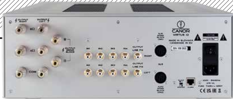
ABOVE: Four line ins and one fixed line out on RCAs are joined by balanced XLR ins for use in mono mode. The 4mm speaker terminals are routed via 8 and 4ohm taps
